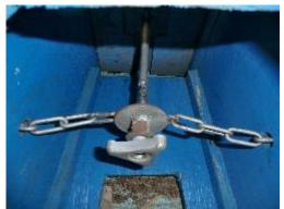
The results are that the components are securely locked together yet store flat when disassembled. Both designs work but the Mark Two is clearly better. Just as when towing, it is a good idea to retighten the bolt after a few minutes of working. Those access ports make this WAY easier than removing the anvil and flipping the stand over something that is needed in the Mark One (though ports could be added if I got around to it).
