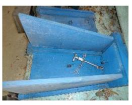
A chain system was cobbed together from a discarded office chair. One link was attached to the end of a long bolt and hands from the downward facing hook (under the top). There is a washer with two chains that hook over the lateral hooks and a large "wing nut" that threads onto the bolt. When the chains are hooked up, the nut is screwed upwards and all componets are locked together.
