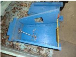
Each chain is inserted through the hole to the outside with sufficient slack to allow the last link to be rotated and used as a lock point.
